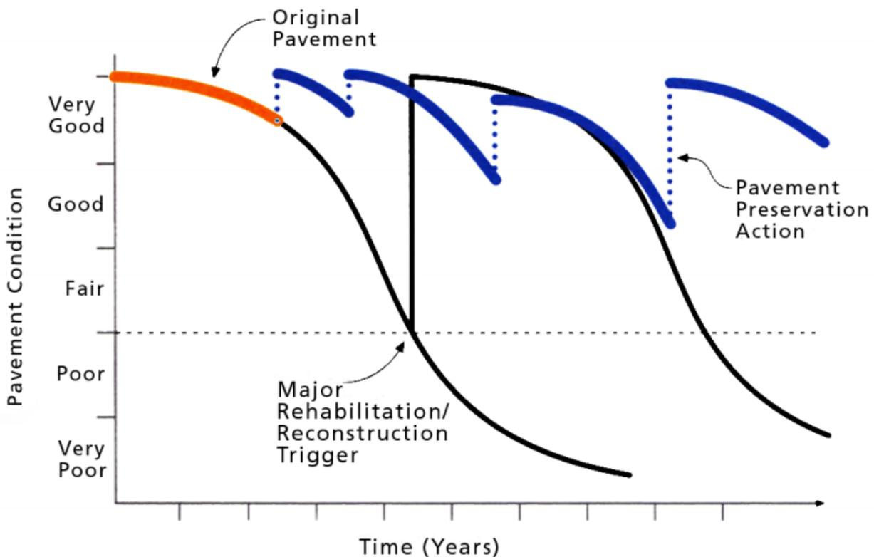
Pavement performance curves are non-linear and once the pavement condition is reduced deterioration accelerates exponentially as shown above.
